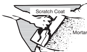
Figure 5 Apply mortar using a plasterer's trowel.
